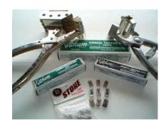
Revolving Head Tattoo with positive Ear release to prevent blurring and scratching. Holds 4 digits on each side, outfit consists of pliers, set of 10mm 0-9 digits and paste
